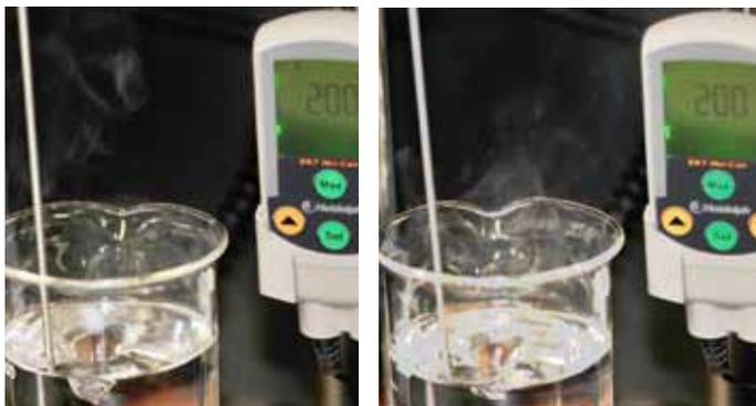
Figure 3: When heated to 200°C, Shell Risella X 415 oils fumes less than Group II conventional oils. The oils used have comparable viscosities to each other at 40°C.
